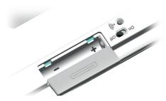
2. Place the 2 AAA-size rechargeable batteries in the battery compartment.
