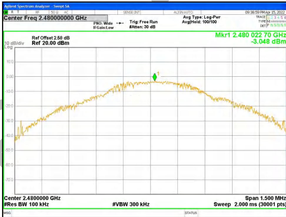
Tx. Spurious NVNT 1-DH1 2480MHz Ant1 Emission
