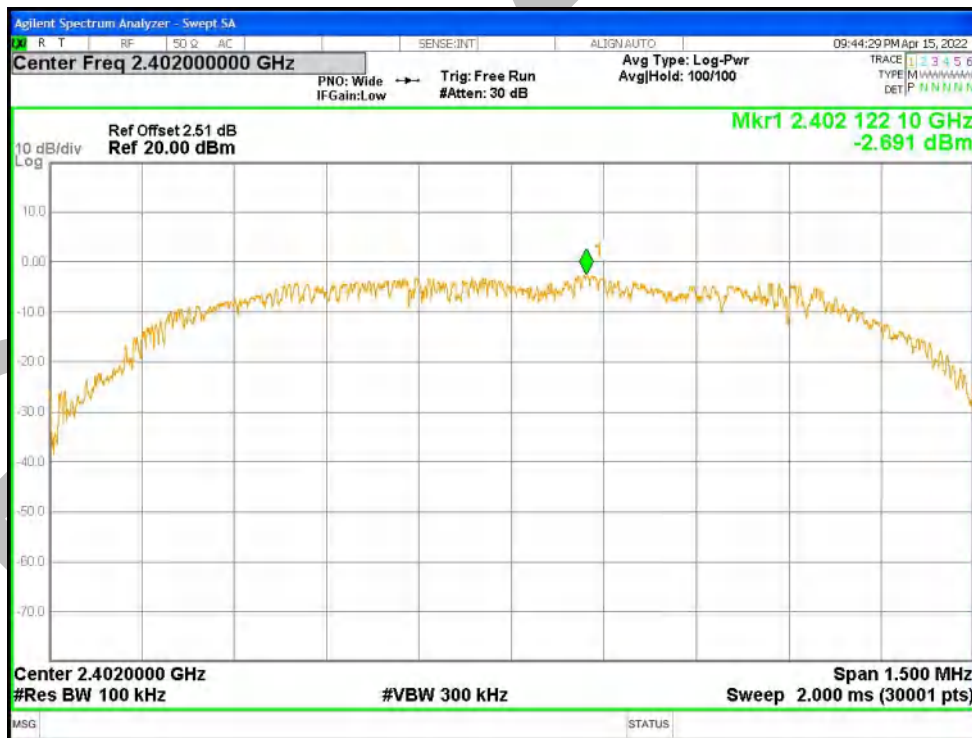
Tx. Spurious NVNT 3-DH1 2402MHz Ant1 Emission
