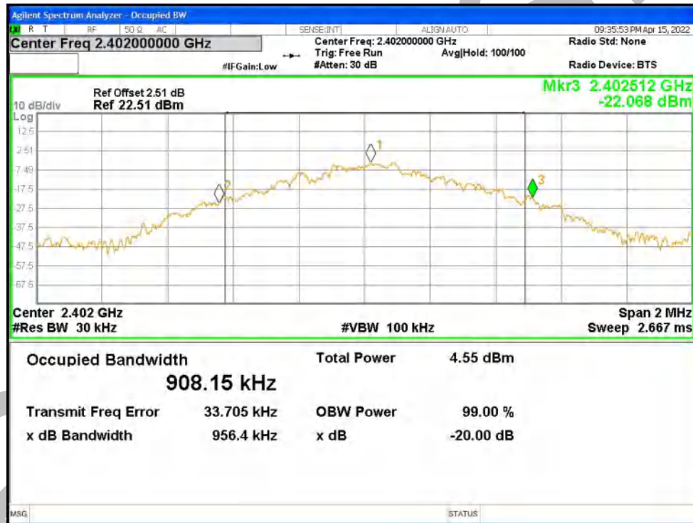
-20dB Bandwidth NVNT 1-DH1 2441MHz Ant1
