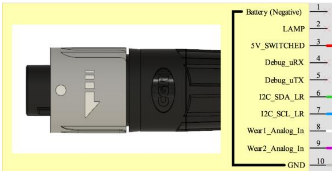
Figure 3 - Sensor Node External Connector Pinouts
