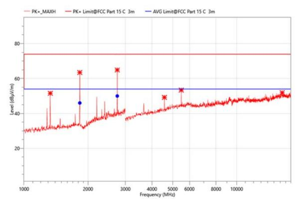
Site: Antenna::Horizontal Temperature(C):23(C) LAB Limit: FCC Part 15 C 3m Radiation **Humidity(%):25% Test Time: EUT: Photoelectric Smoke Alarm** 2023-08-23 DC 3V M/N.: **S1-R Power Rating: Test Engineer:** Mode: TXVier Note:
