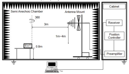
$$10\ {\rm of}$$  (c) Radiated Emission Test Set-Up, Frequency Above 1000MHz
