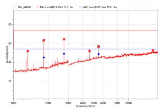
Site: LAB Antenna::Vertical **Temperature(C):23(C) Humidity(%):25%** FCC Part 15 C 3m Radiation Limit: 2023-08-23 EUT: **Photoelectric Smoke Alarm Test Time:** M/N.: S1-R **Power Rating:** DC 3V Mode: TX**Test Engineer:** Vier Note:
