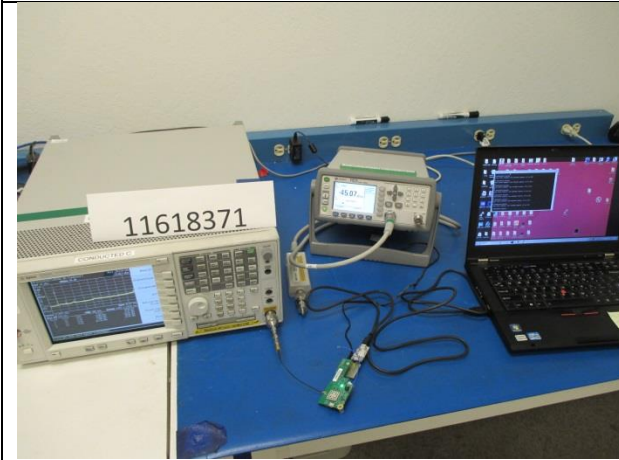
ANTENNA PORT CONDUCTED PHOTO
