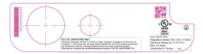
Location of FCC ID label: The above FCC ID label is placed on the bottom of EUT
