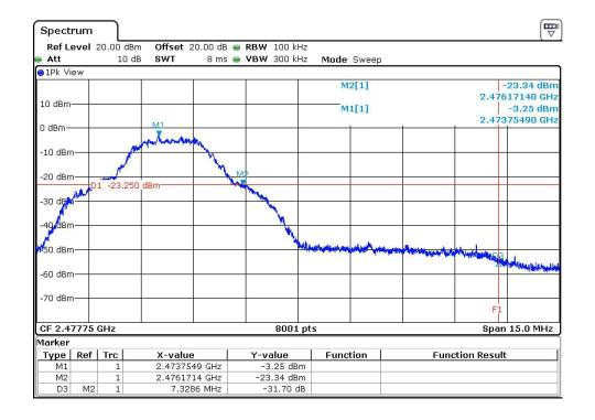
DTS bandwidth measurement procedure
