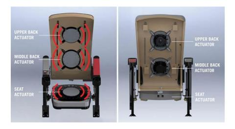
controls; electronics governing the operation of the chairs; a server, Tremor FX Processor or wireless transmitter; and software.
