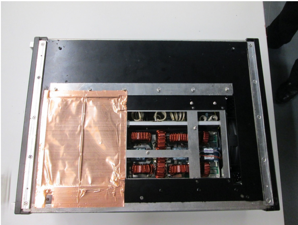
Photo A3-3: copper foil on bottom
