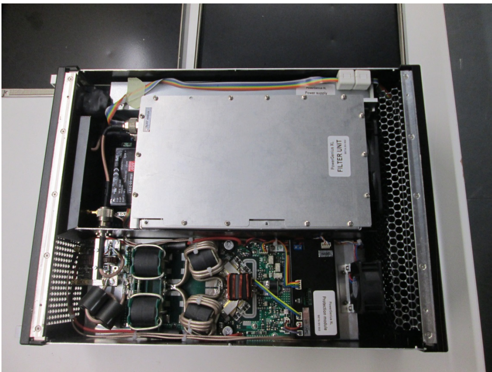
Photo A3-5: ferrite on display line
