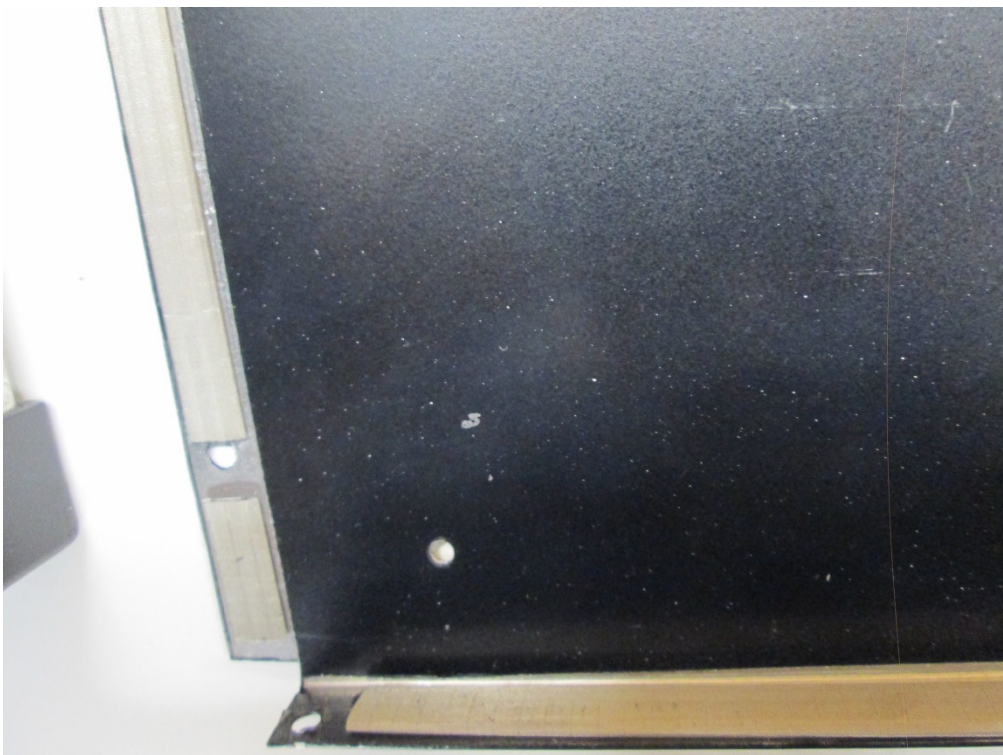
Photo A3-2: top, bottom and front bonded with EMC gaskets
