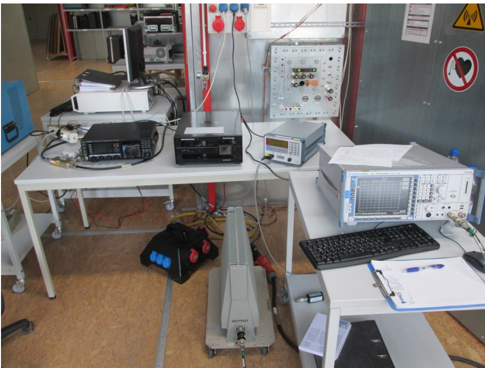
Photo A1-4 spurious emissions and gain measurement
