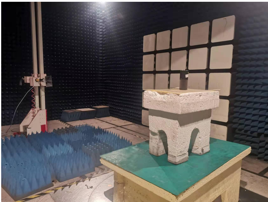
Spurious Emission Test Setup (Above 1GHz)
