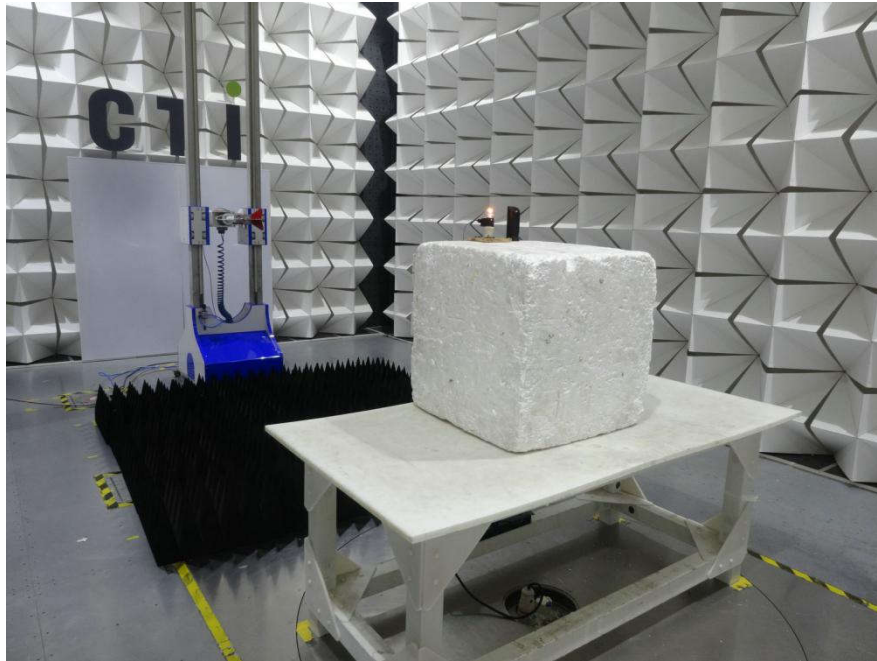
Radiated spurious emission Test Setup-3(Above 1GHz)
