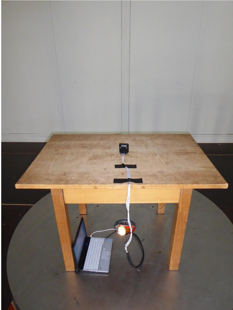
172200_11: Test setup open area test site M6, 30 MHz – 1 GHz
