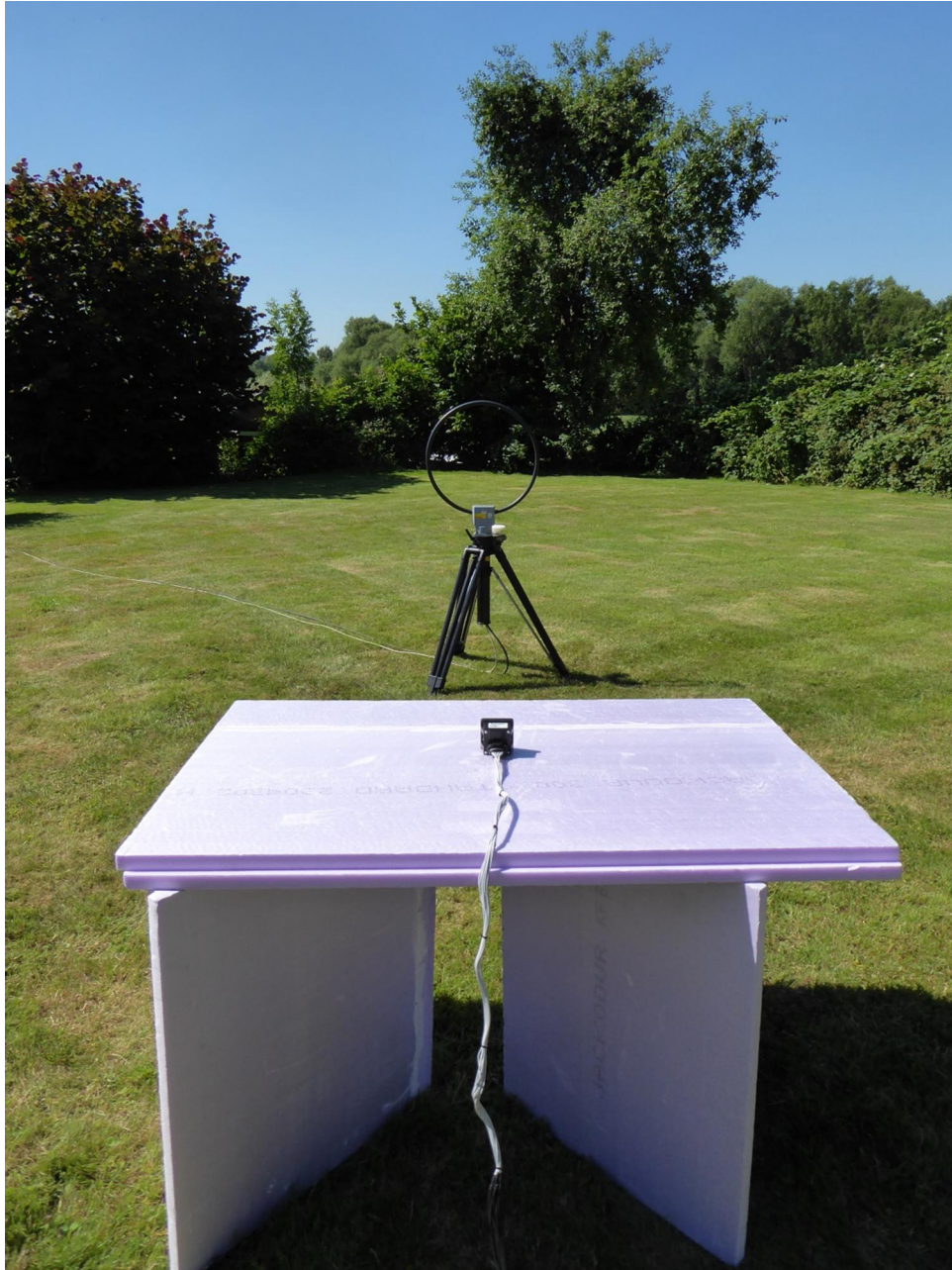
172200_06: Test setup open area test site, 9 kHz – 30 MHz @ 3m
