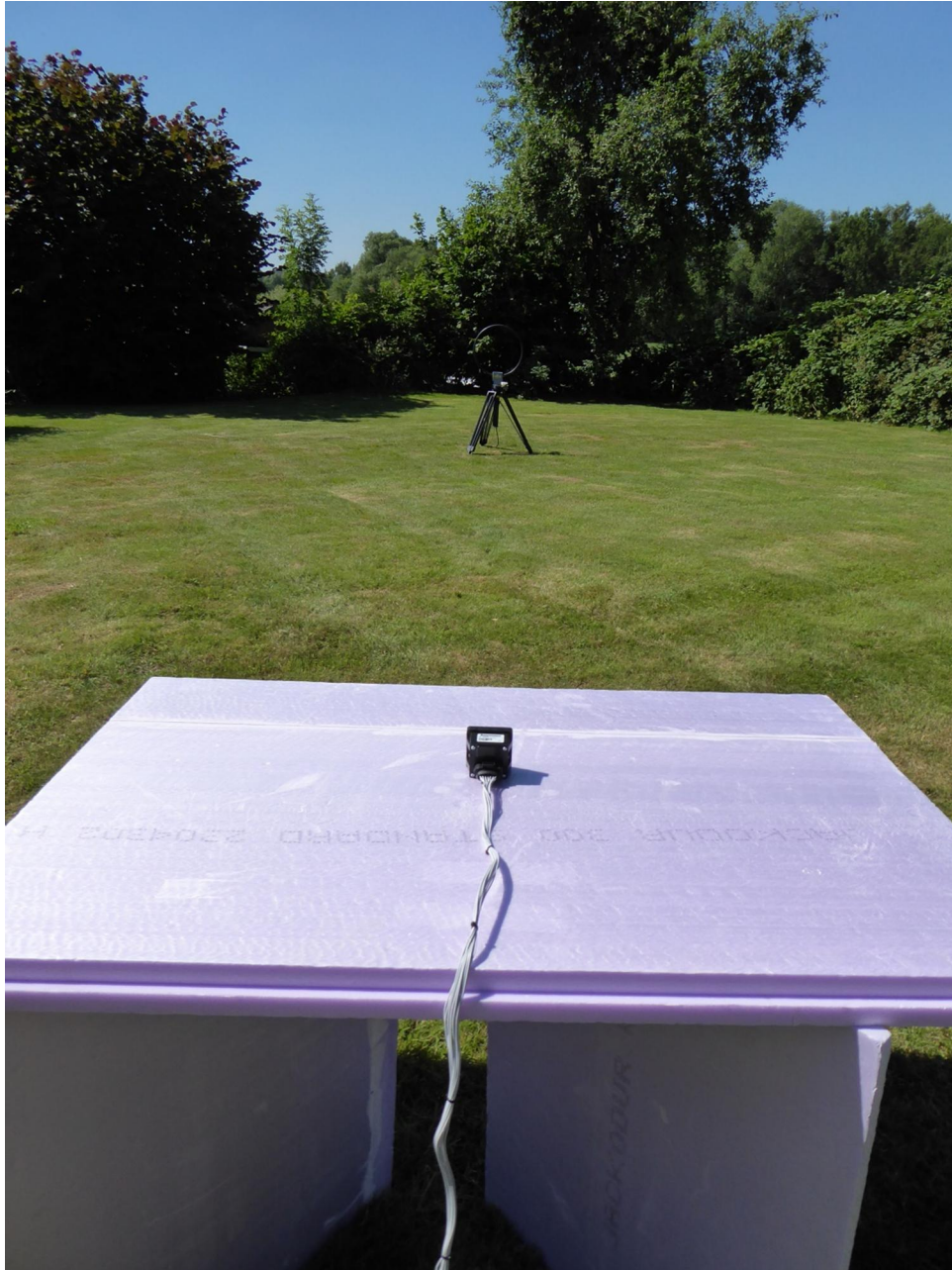
172200_08: Test setup open area test site, 9 kHz – 30 MHz @ 10m
