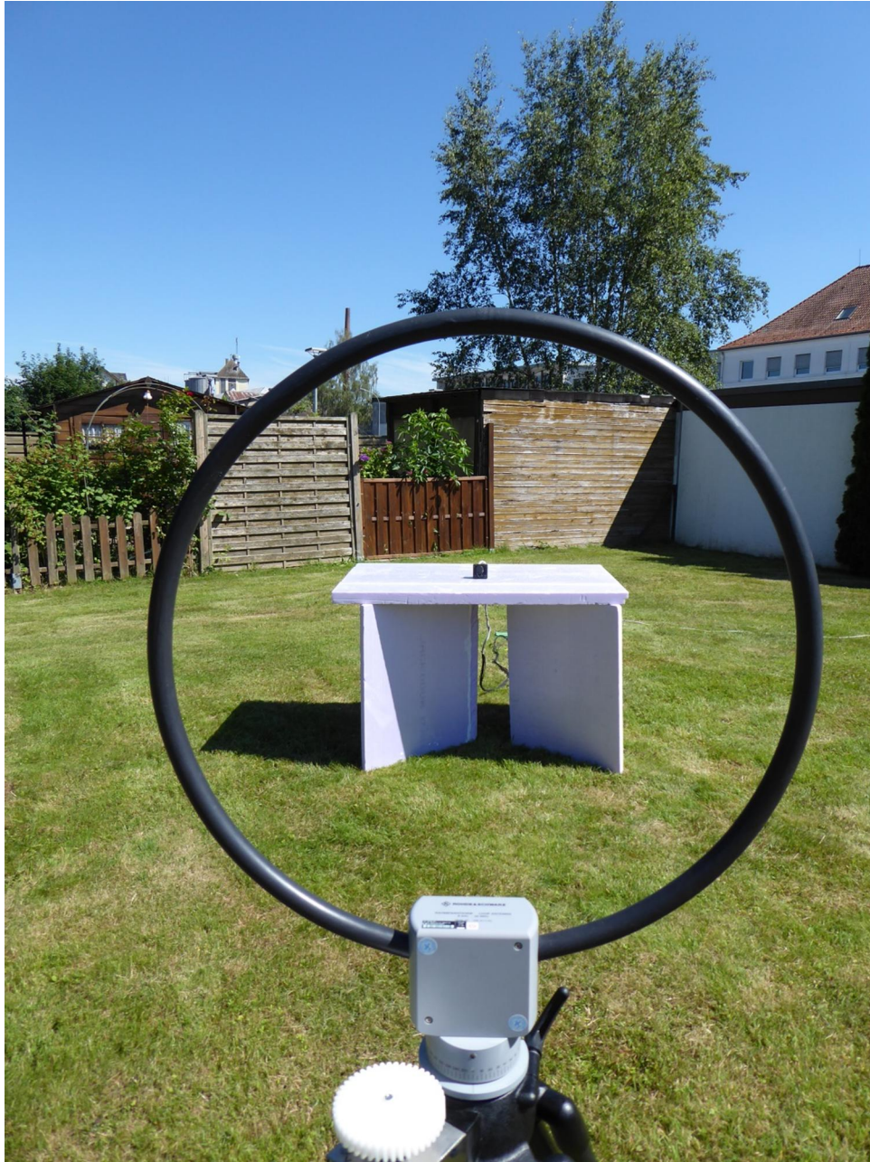
172200_05: Test setup open area test site, 9 kHz – 30 MHz @ 3m
