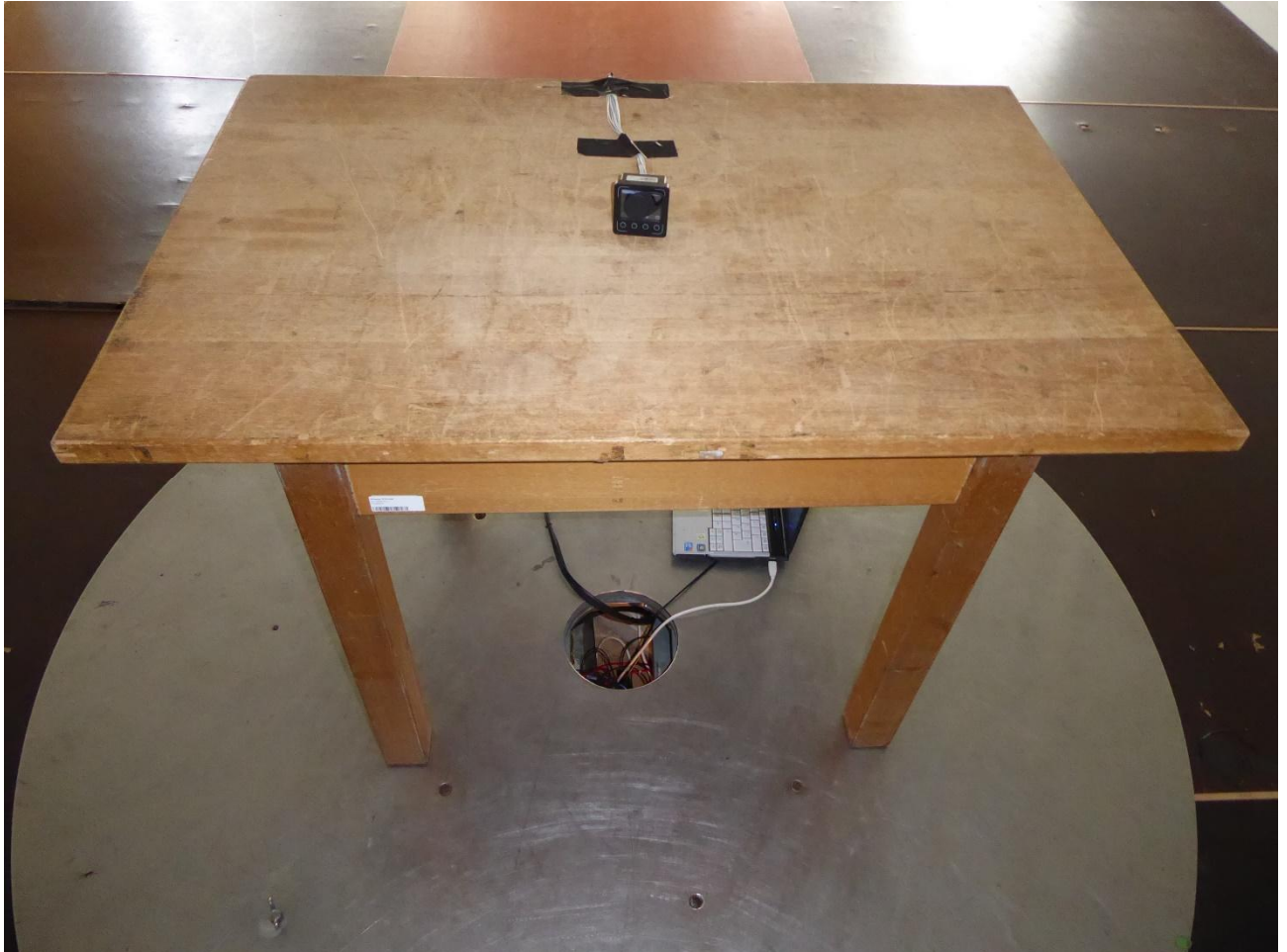
172200_10: Test setup open area test site M6, 30 MHz – 1 GHz
