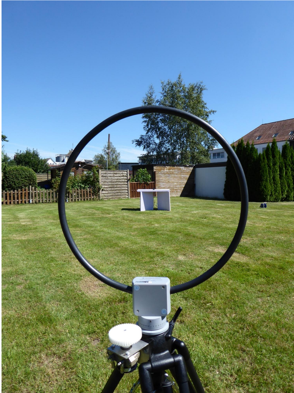
172200_07: Test setup open area test site, 9 kHz – 30 MHz @ 10m
