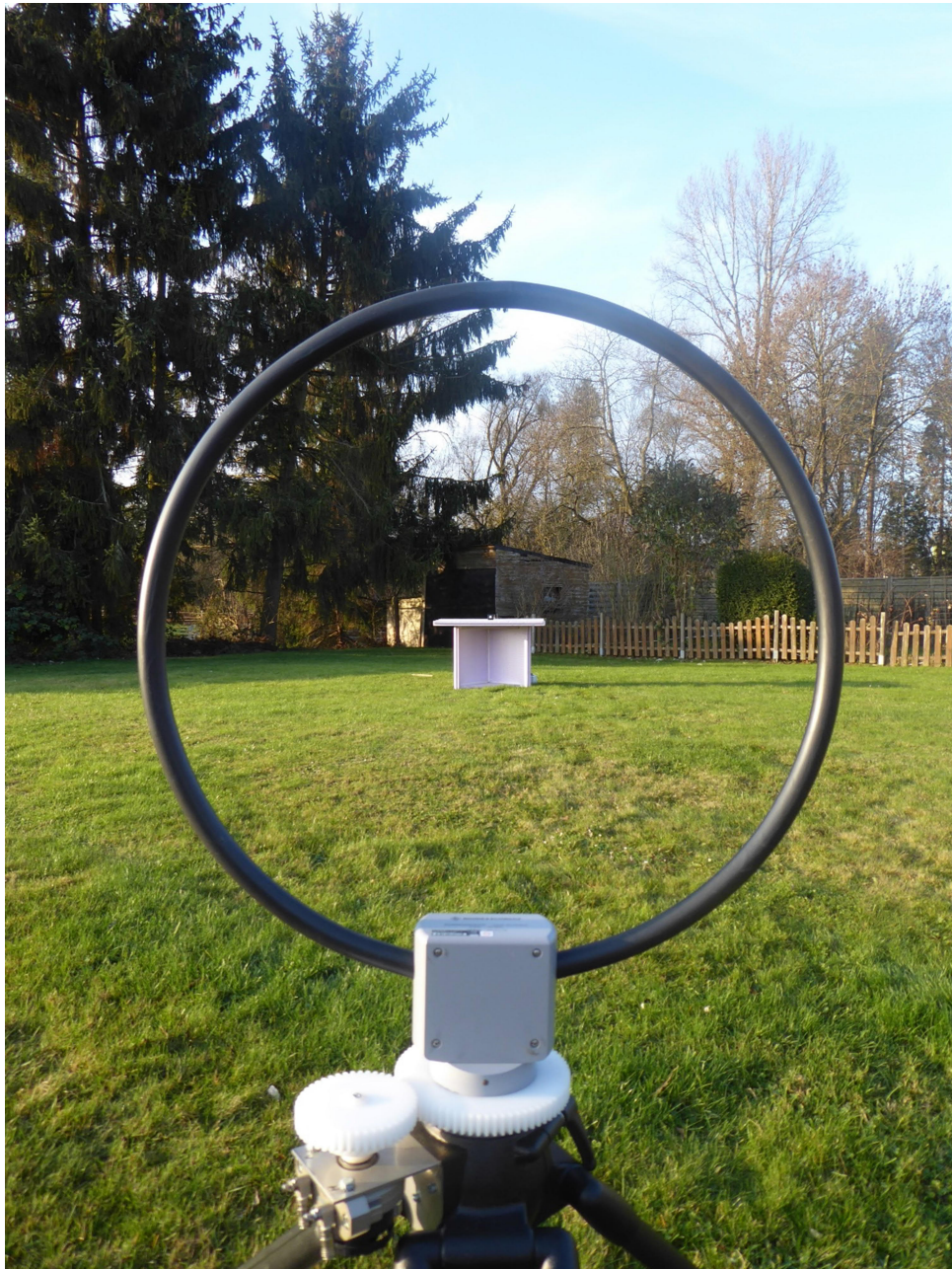
Test setup OATS; Final measurement 9 kHz to 30 MHz
