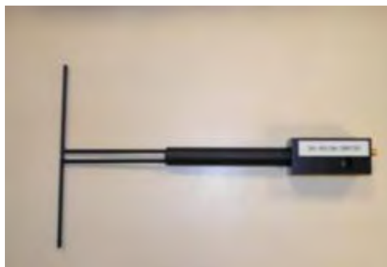
Figure 1 – MVG COMOSAR Validation Dipole
