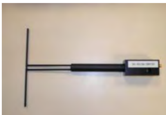
Figure 1 – MVG COMOSAR Validation Dipole
