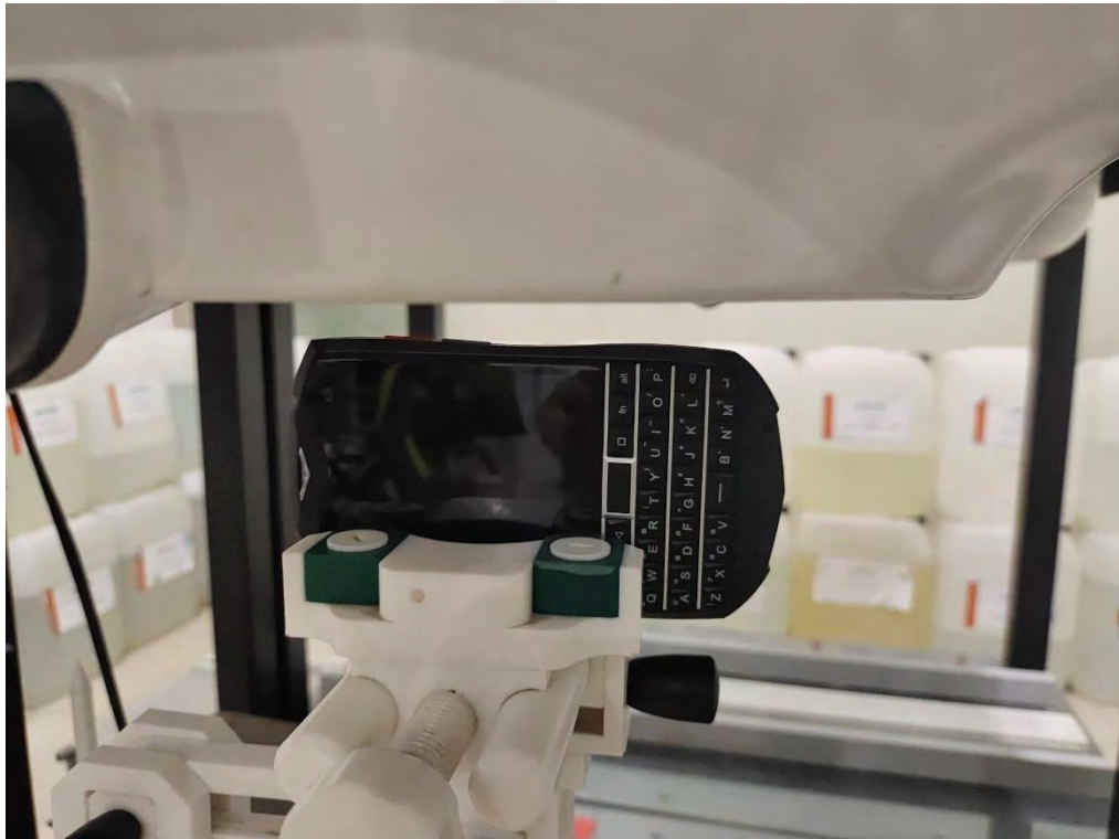
Body Right side(separation distance is 10mm)
