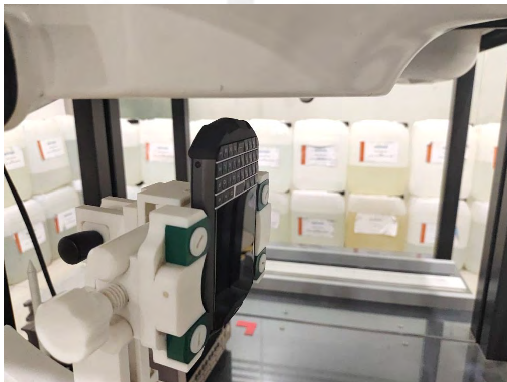
Body Top side(separation distance is 10mm)
