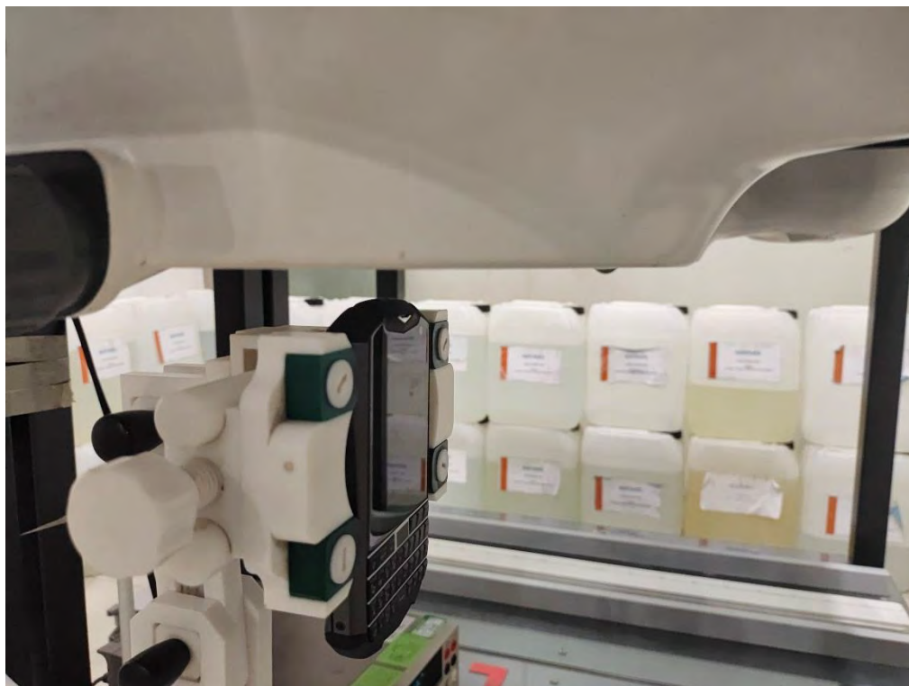
Body Bottom side(separation distance is 10mm)
