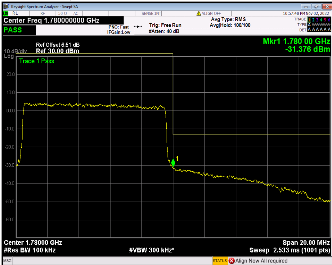
Band66 QPSK BW=15MHz Channel=132047 RB Size=75 Position=#0
