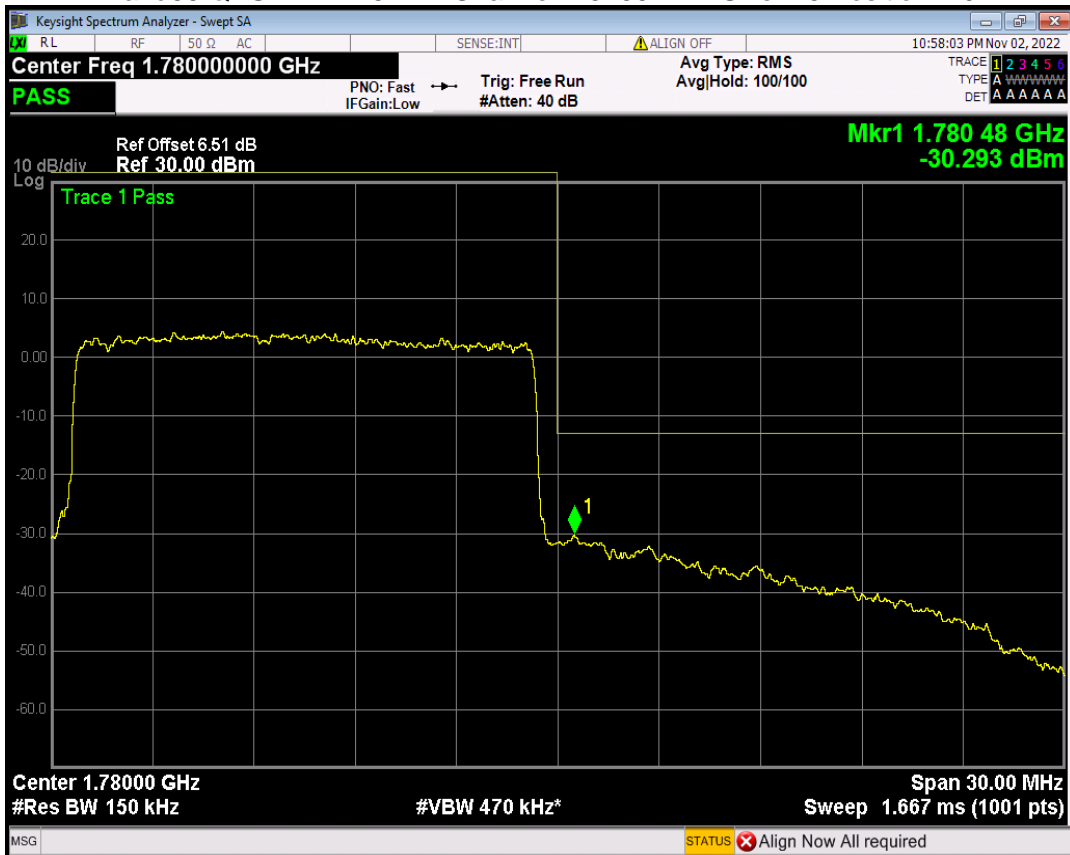
Band66 QPSK BW=20MHz Channel=132072 RB Size=100 Position=#0
