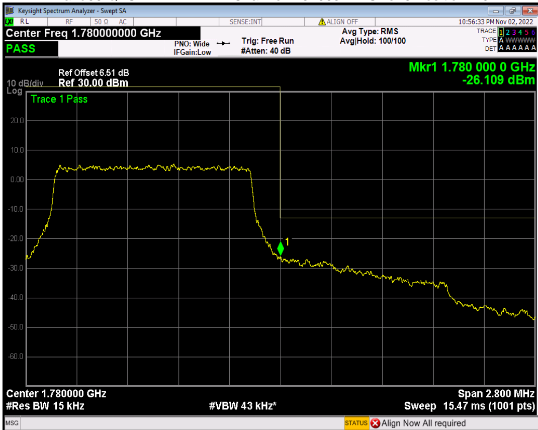
Band66 QPSK BW=10MHz Channel=132022 RB Size=50 Position=#0
