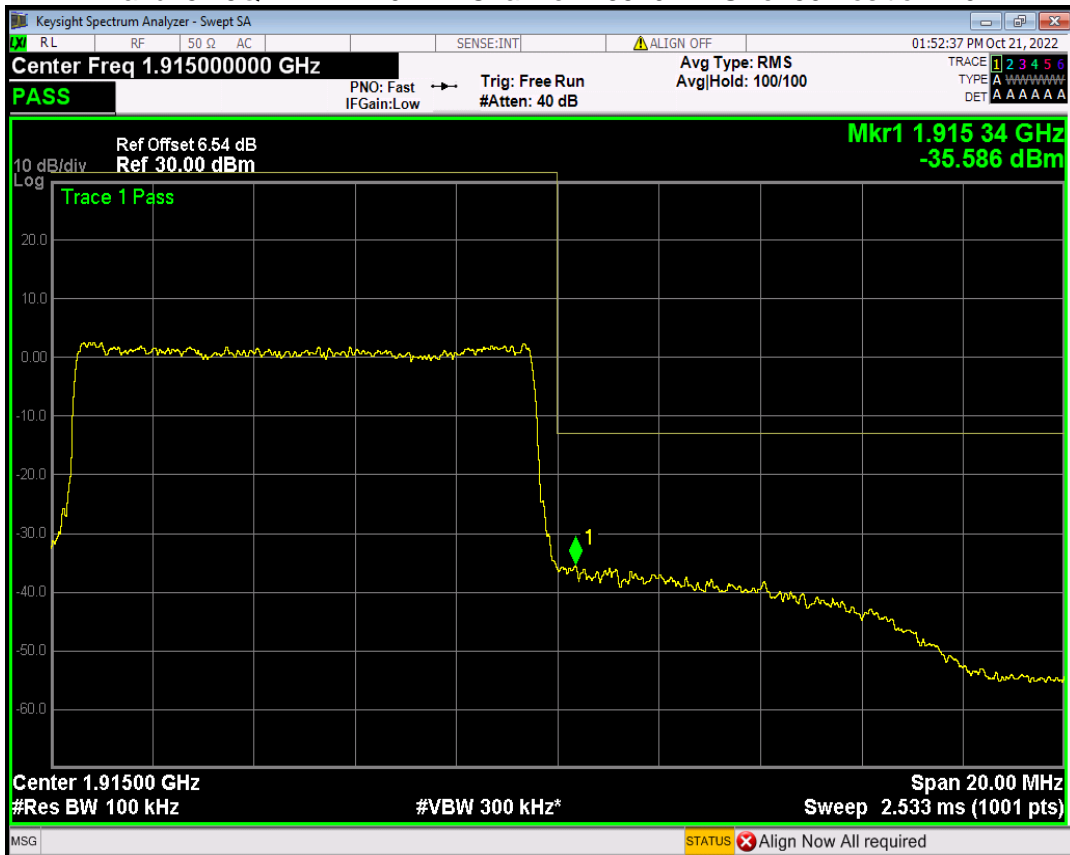
Band25 16QAM BW=15MHz Channel=26115 RB Size=75 Position=#0
