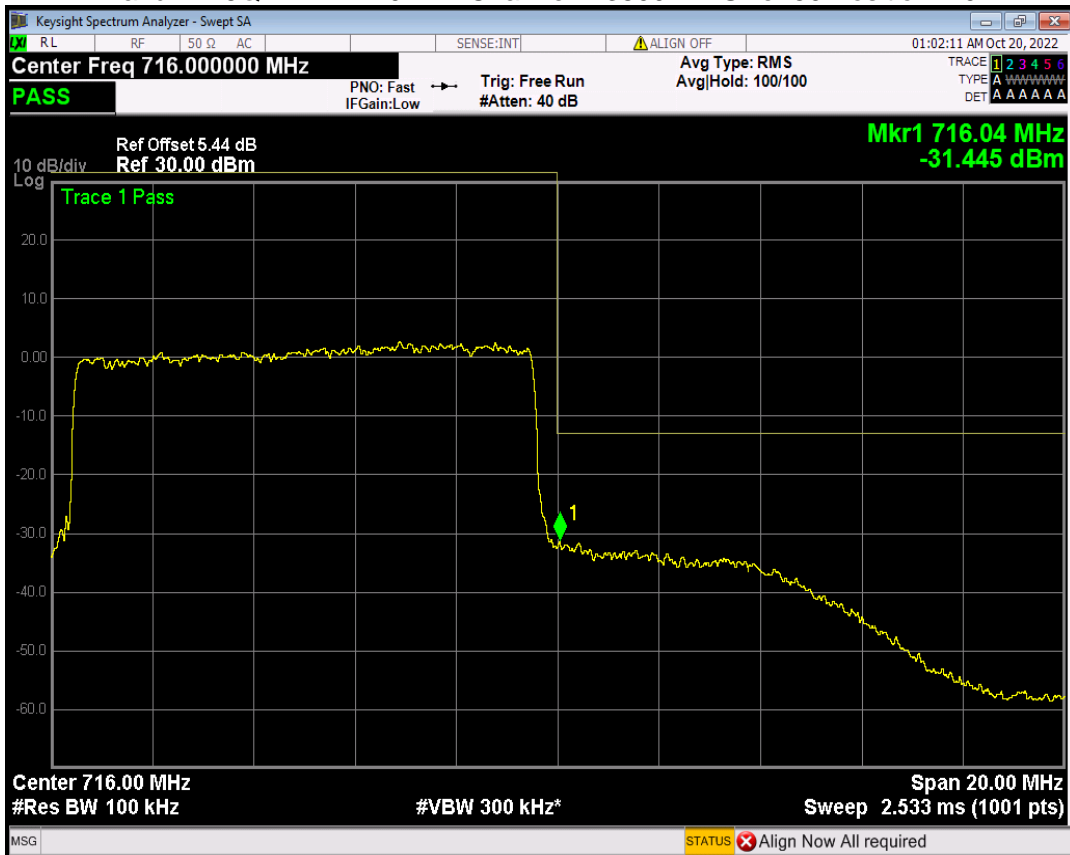
Band17 16QAM BW=5MHz Channel=23755 RB Size=25 Position=#0
