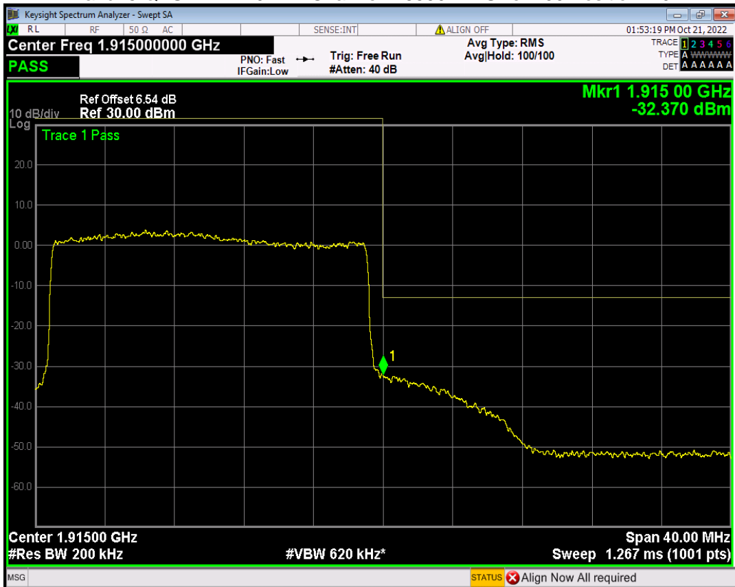
Band25 QPSK BW=3MHz Channel=26055 RB Size=15 Position=#0
