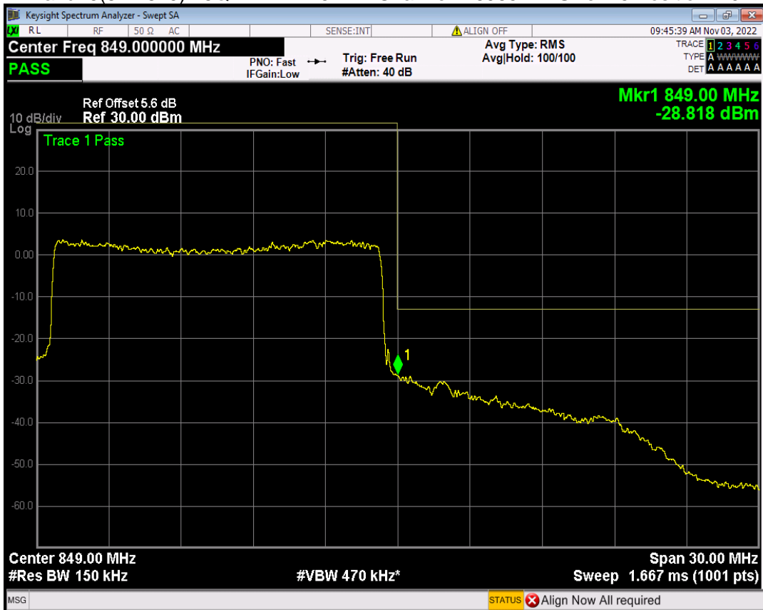
Band26(824-849) 16QAM BW=3MHz Channel=26805 RB Size=15 Position=#0
