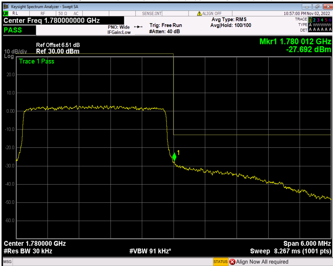
Band66 16QAM BW=5MHz Channel=131997 RB Size=25 Position=#0
