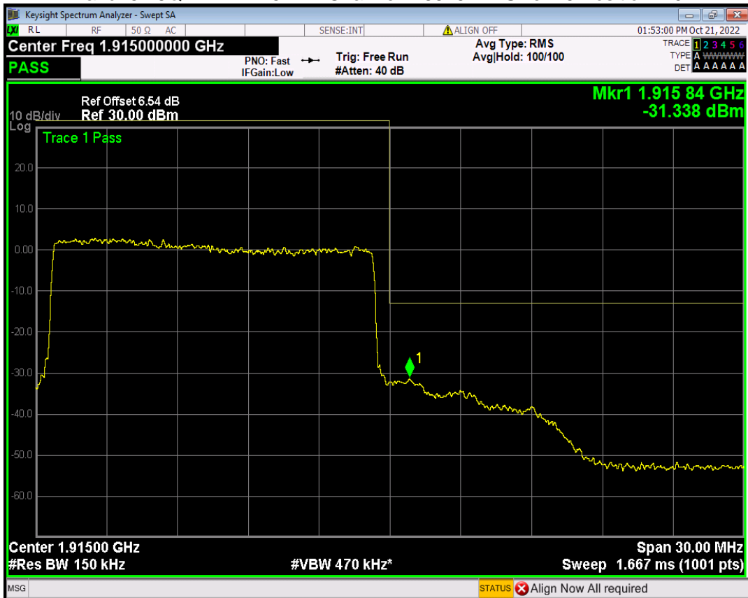
Band25 16QAM BW=20MHz Channel=26140 RB Size=100 Position=#0
