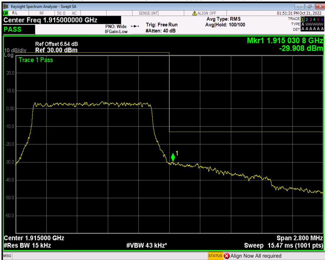
Band25 QPSK BW=10MHz Channel=26090 RB Size=50 Position=#0
