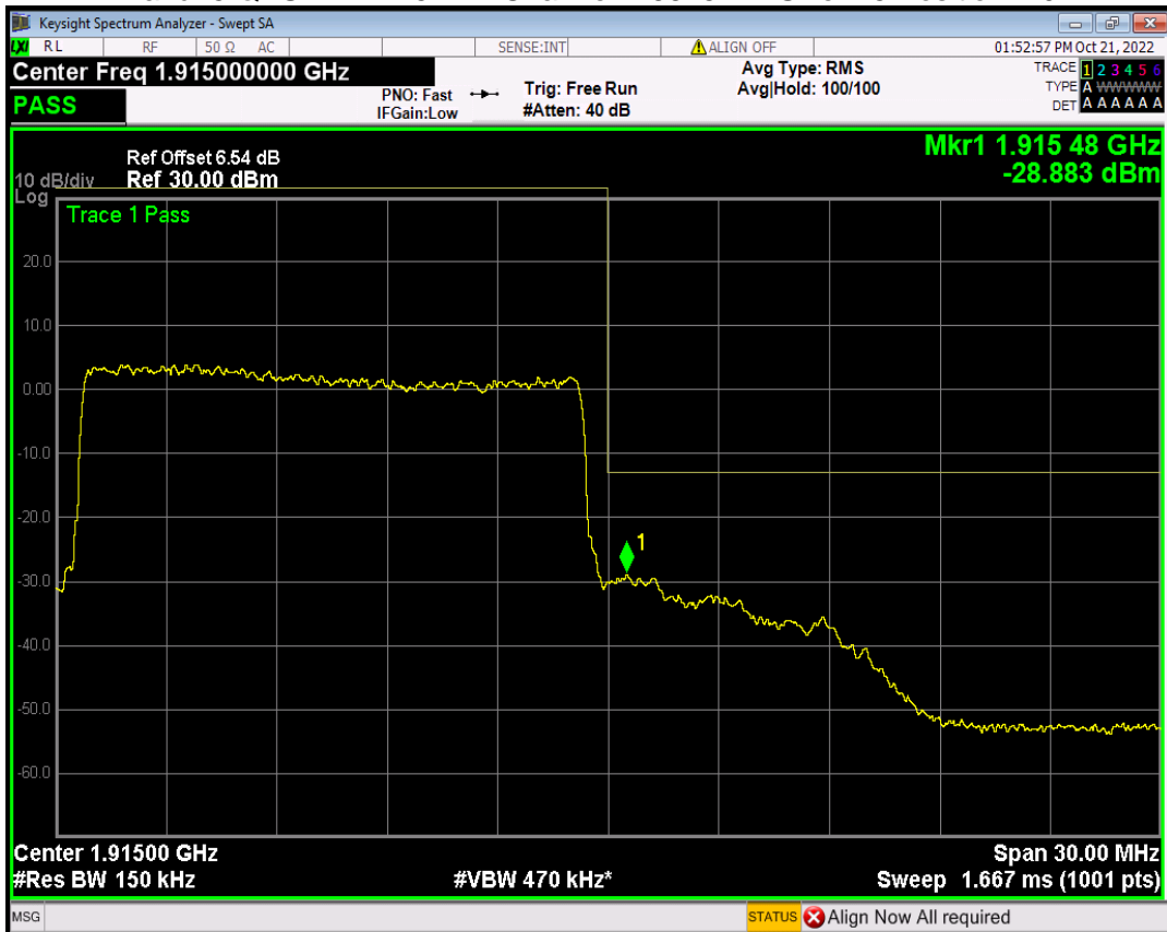
Band25 QPSK BW=20MHz Channel=26140 RB Size=100 Position=#0
