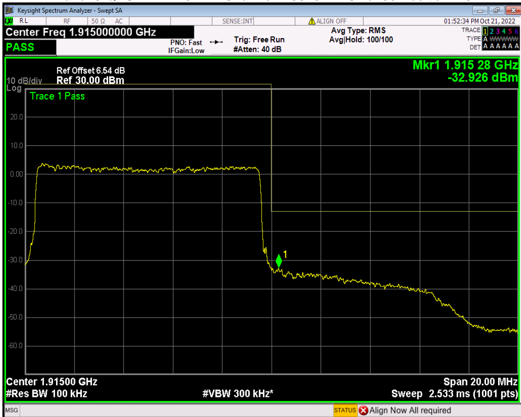
Band25 QPSK BW=15MHz Channel=26115 RB Size=75 Position=#0
