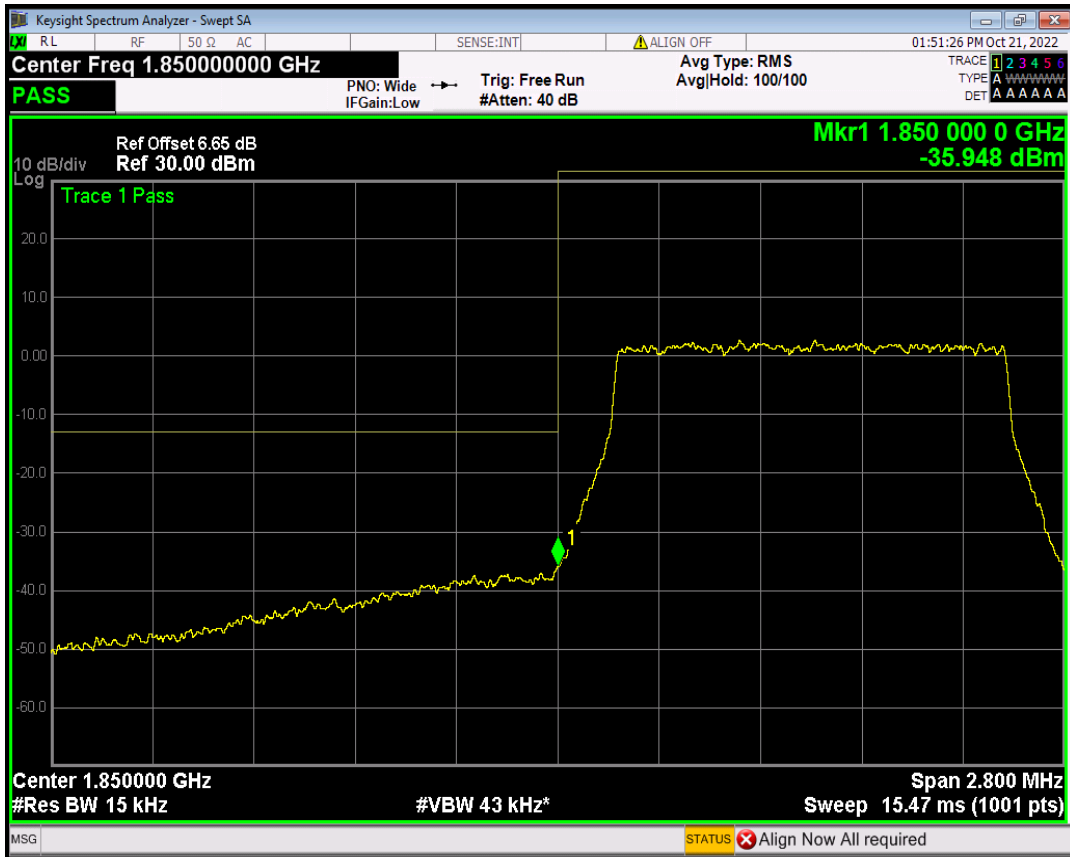
Band25 16QAM BW=1.4MHz Channel=26683 RB Size=6 Position=#0
