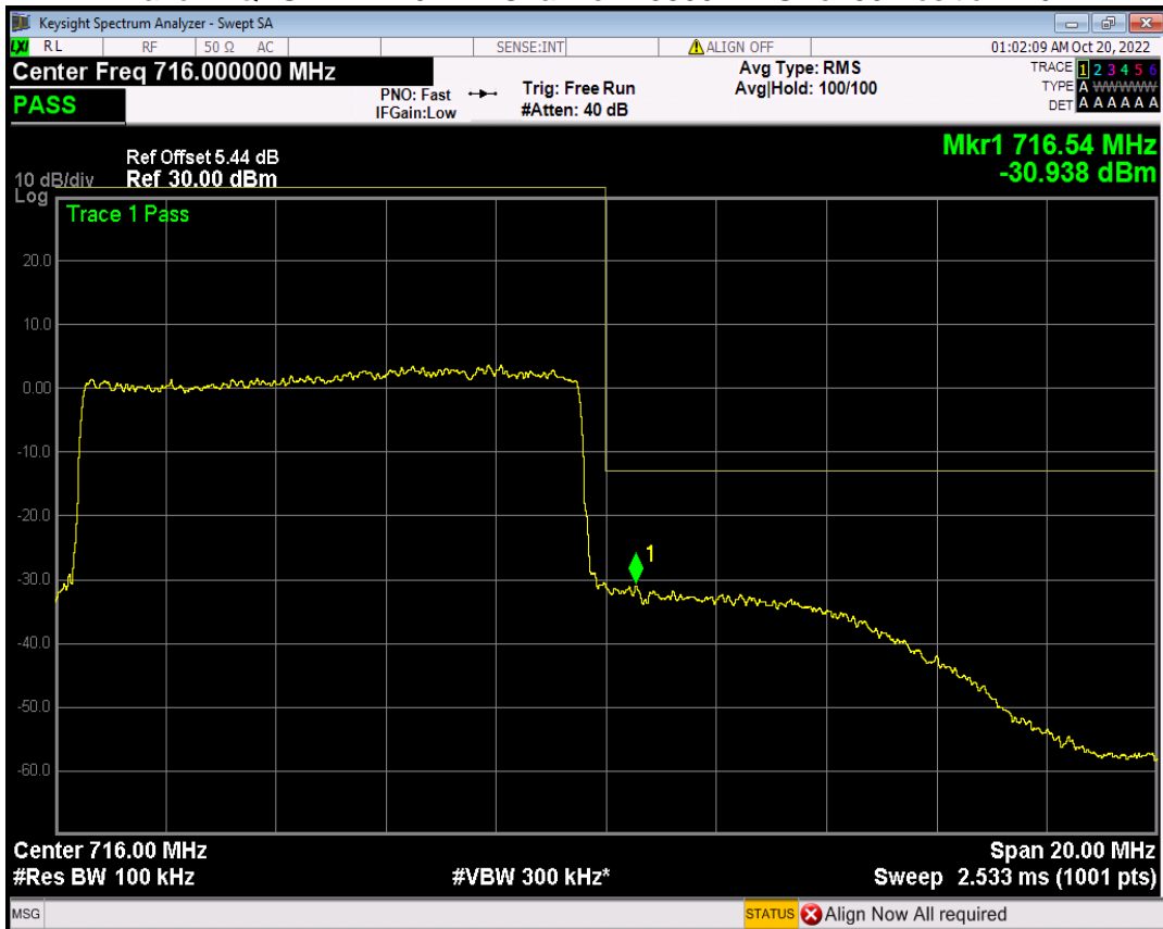
Band17 QPSK BW=5MHz Channel=23755 RB Size=25 Position=#0
