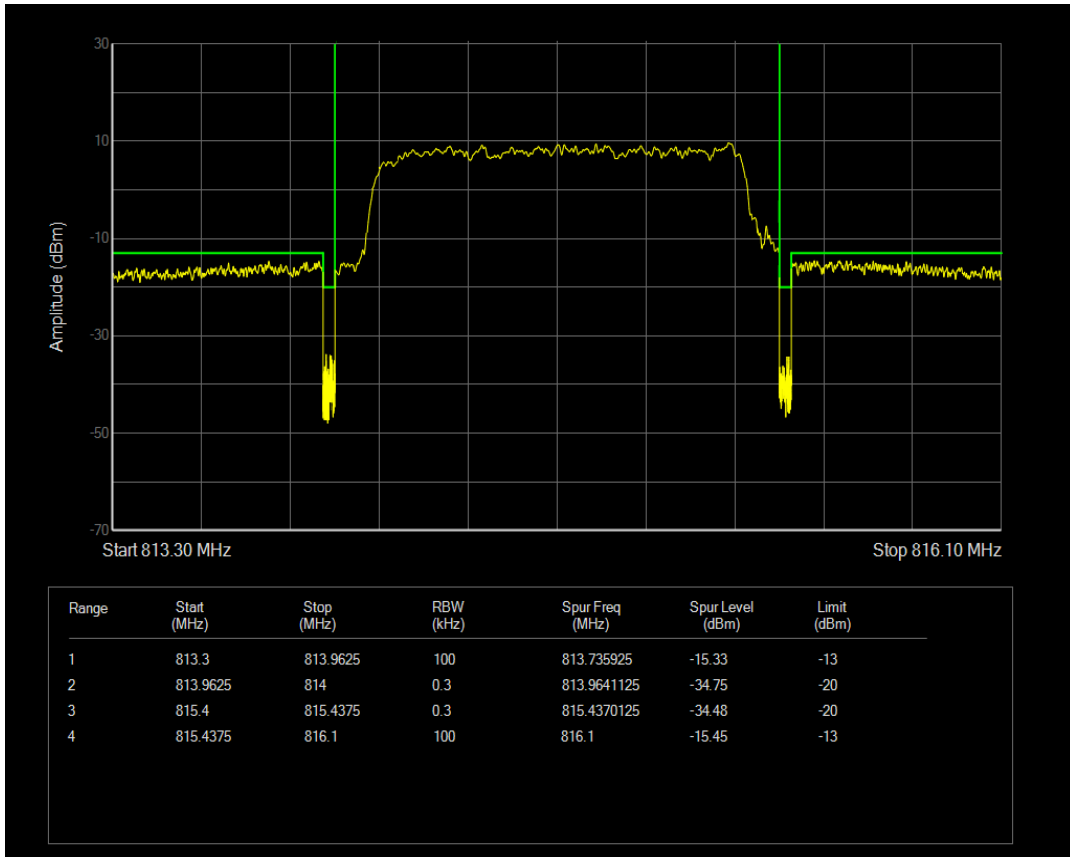
Band26(814-824) QPSK BW=1.4MHz Channel=26783 RB Size=6 Position=#0
