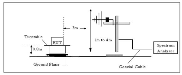
(A) Radiated Emission Test-Up Frequency 30MHz~1GHz
