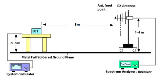
For radiated test from above 1GHz
