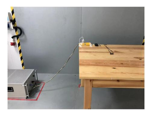
Radiated Emission Test Setup Photo - Below 1GHz
