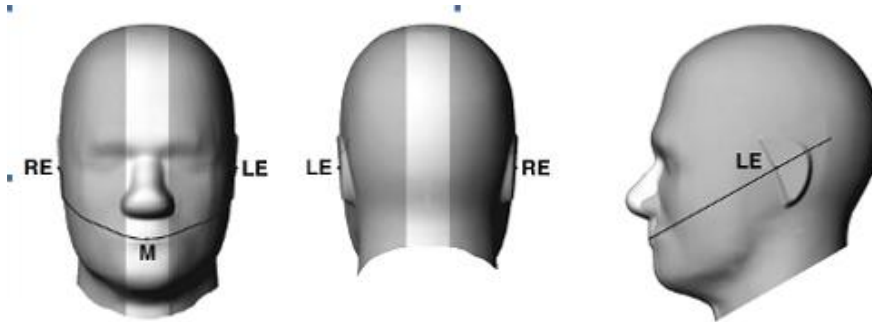
F-3. Front, back, and side views of SAM (model for the phantom shell). Full-head model is for illustration purposes only-procedures in this recommended practice are intended primarily for the phantom setup.
