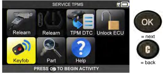
Depending on the make and model of the selected vehicle, the VT57 asks you to choose the communication frequency for the key fob being tested.
