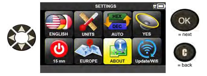
The **About** screen is displayed. This displays the VT57 serial number, the firmware and database version numbers and the validity of the user licence.
