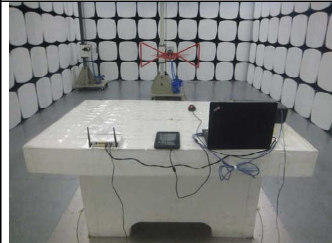
Radiated Emissions Test Setup Below 1GHz
