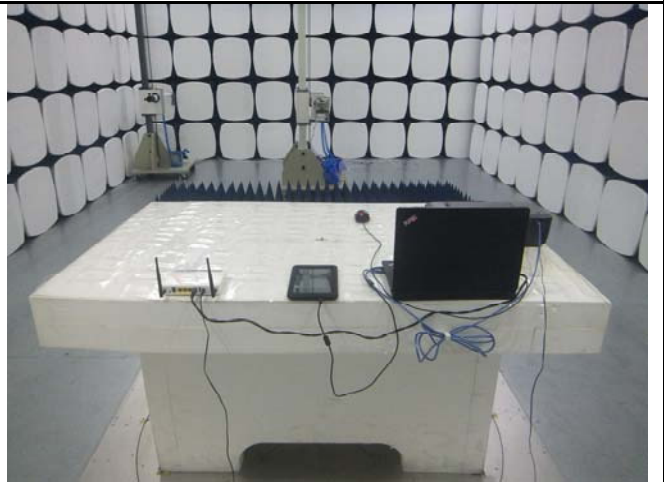
Radiated Emissions Test Setup Above 1GHz
