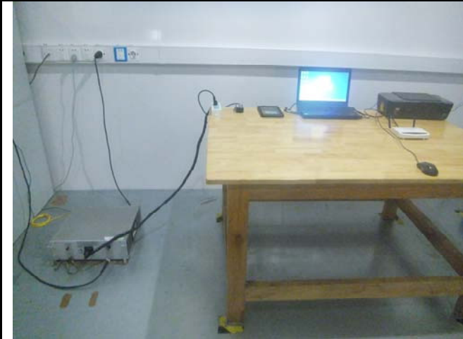
Conducted Emissions Test Setup – Front View
