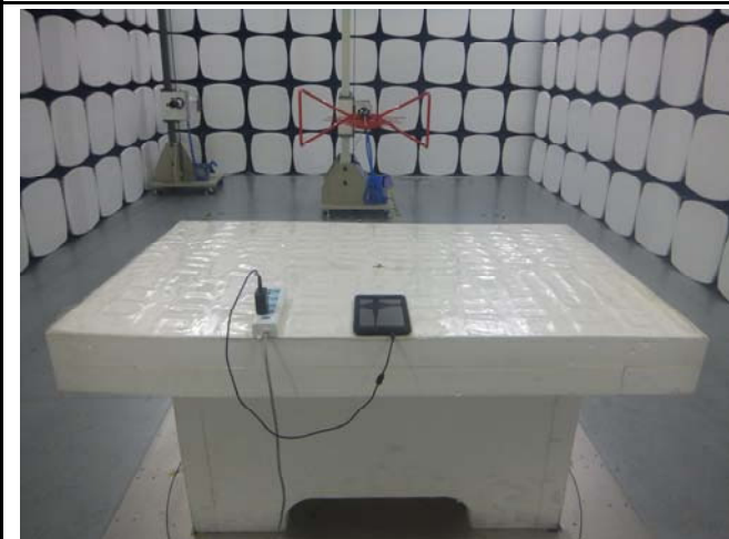
Conducted Emissions Test Setup Front View
