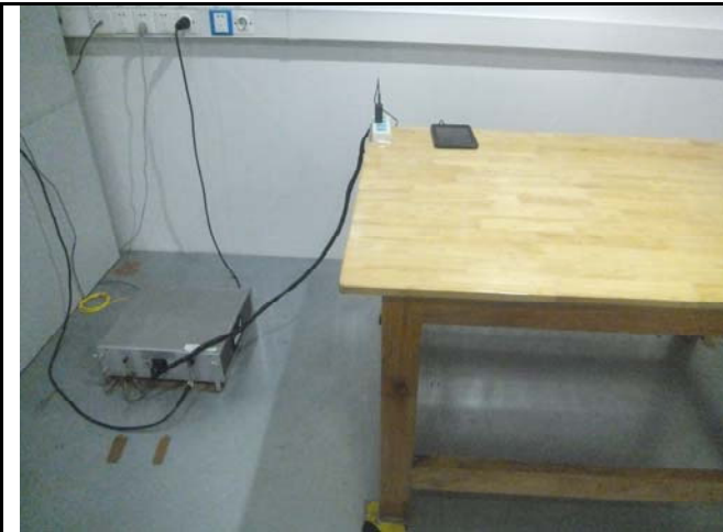
Conducted Emissions Test Setup Front View
