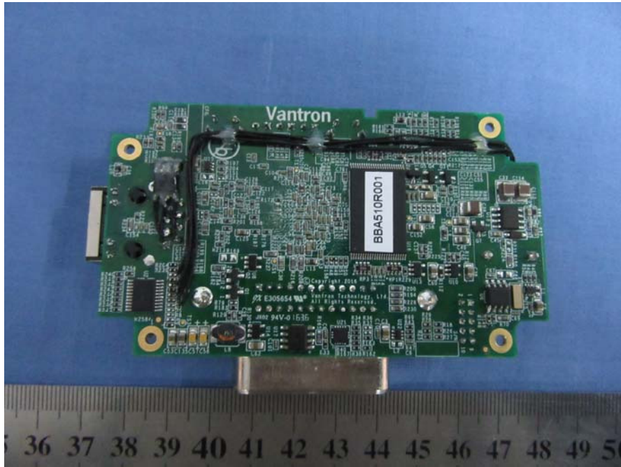
EUT – Main Board Bottom View
