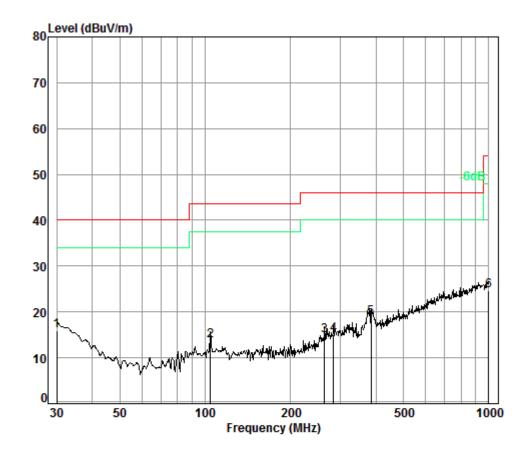
Condition: 3m VERTICAL Job No. : 0236CR Test mode: TX
