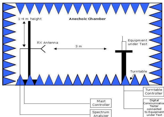
Setup in the Anechoic chamber. For measurements below 1 GHz the ground was replaced by a conducting ground plane.
