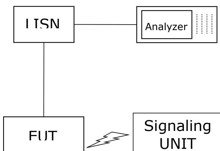
Setup in the shielded room for conducted measurements at AC mains port
