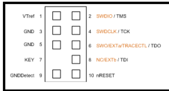
Figure 2. 10-Pin Cortex Debug Connector
