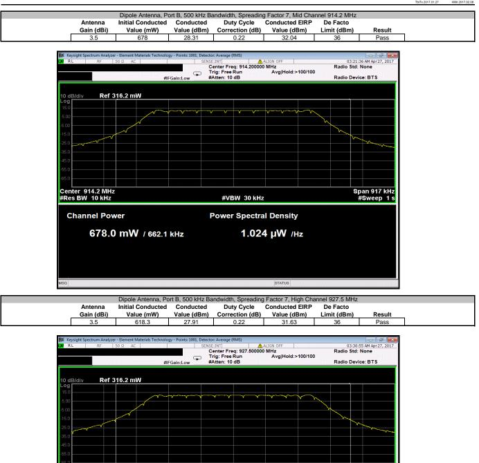
Center 927.5 MHz #Res BW 10 kHz Span 915.1 kHz #Sweep 1 s #VBW 30 kHz **Channel Power Power Spectral Density** 618.3 mW / 660.7 kHz 935.8 nW /Hz
