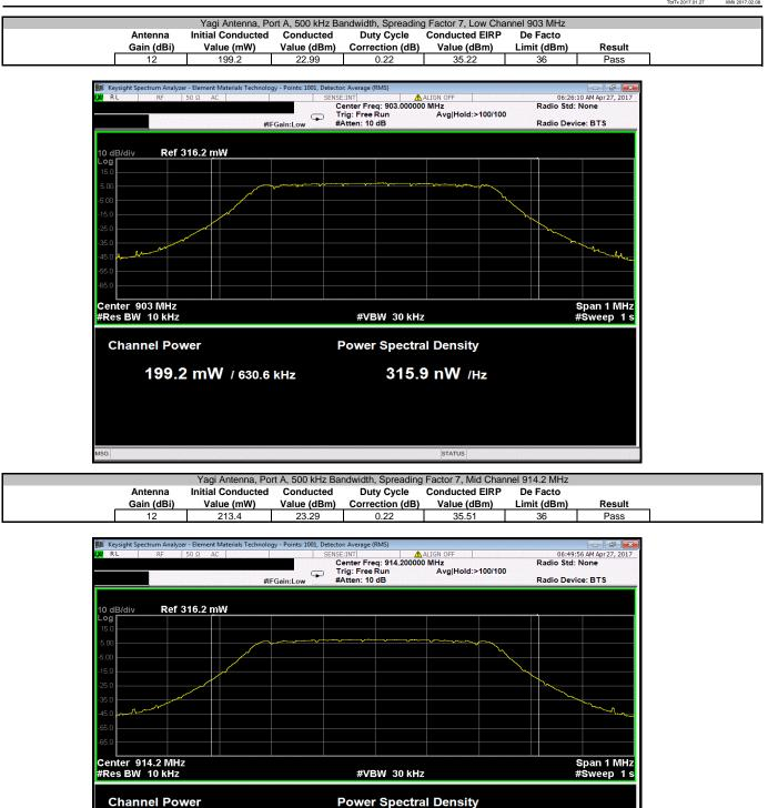
**Channel Power Power Spectral Density** 213.4 mW / 630.5 kHz 338.5 nW /Hz STATUS
