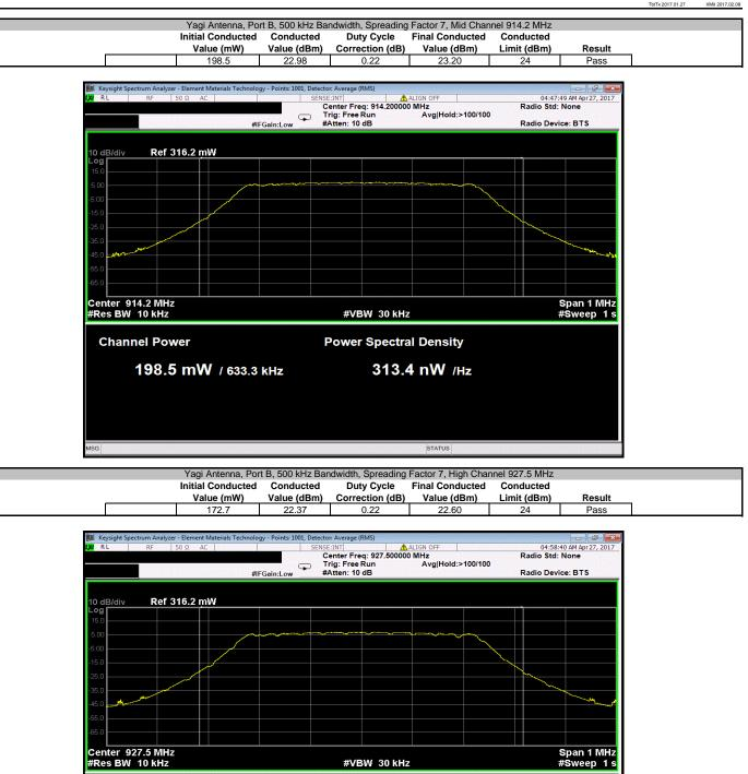
**Channel Power Power Spectral Density** 172.7 mW / 632.9 kHz 272.8 nW /Hz
