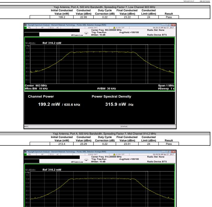
Center 914.2 MHz #Res BW 10 kHz Span 1 MHz #Sweep 1 s #VBW 30 kHz **Channel Power Power Spectral Density** 213.4 mW / 630.5 kHz 338.5 nW /Hz
