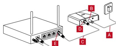
1. As shown, power up the **Cellular Field Station** by connecting the adapter cable (A) to the power jack (B) on the Cellular Field Station, and plug it into an outlet.
