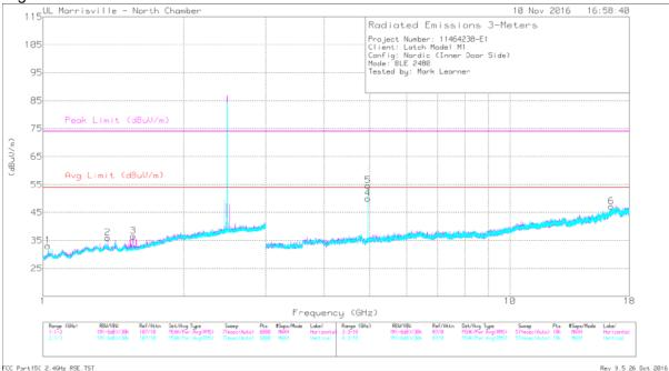
Note: Pre-scan plot taken at 1MHz/30kHz (RBW/VBW). Final measurements taken at 1MHz/3MHz (RBW/VBW).
