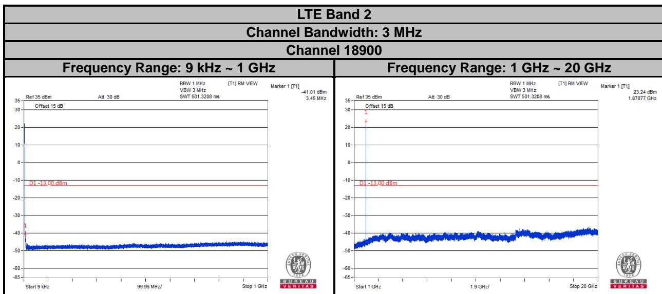
Note: The signal over the limit in 9 kHz is from spectrum analyzer.
