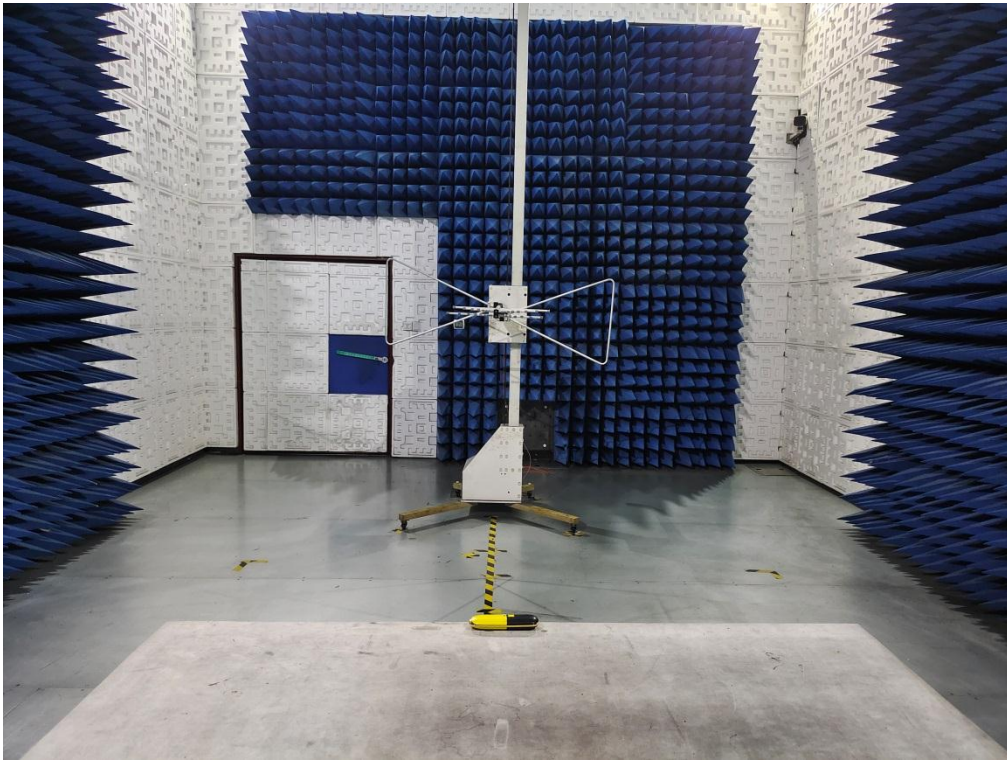
RADIATED EMISSION TEST SETUP ABOVE 1GHZ
