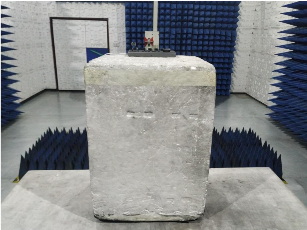
RADIATED EMISSION TEST SETUP ABOVE 1GHz
