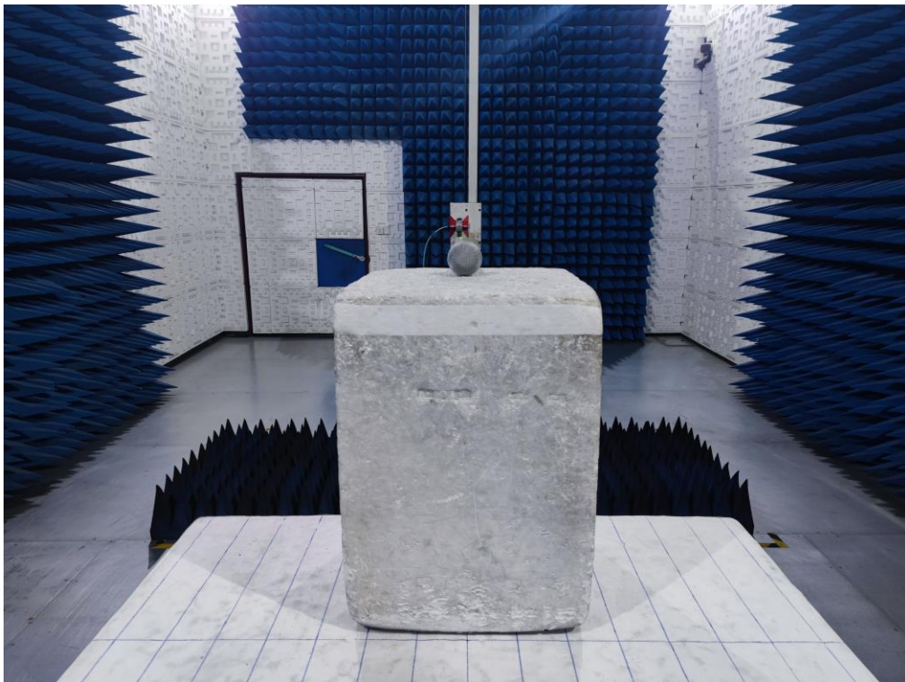
RADIATED EMISSION TEST SETUP ABOVE 1GHz
