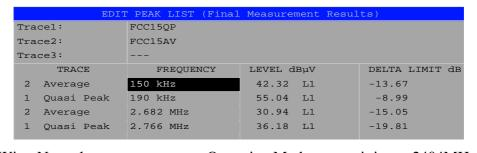
Tested Wire: Neutral Operation Mode: transmitting at 2404MHz
