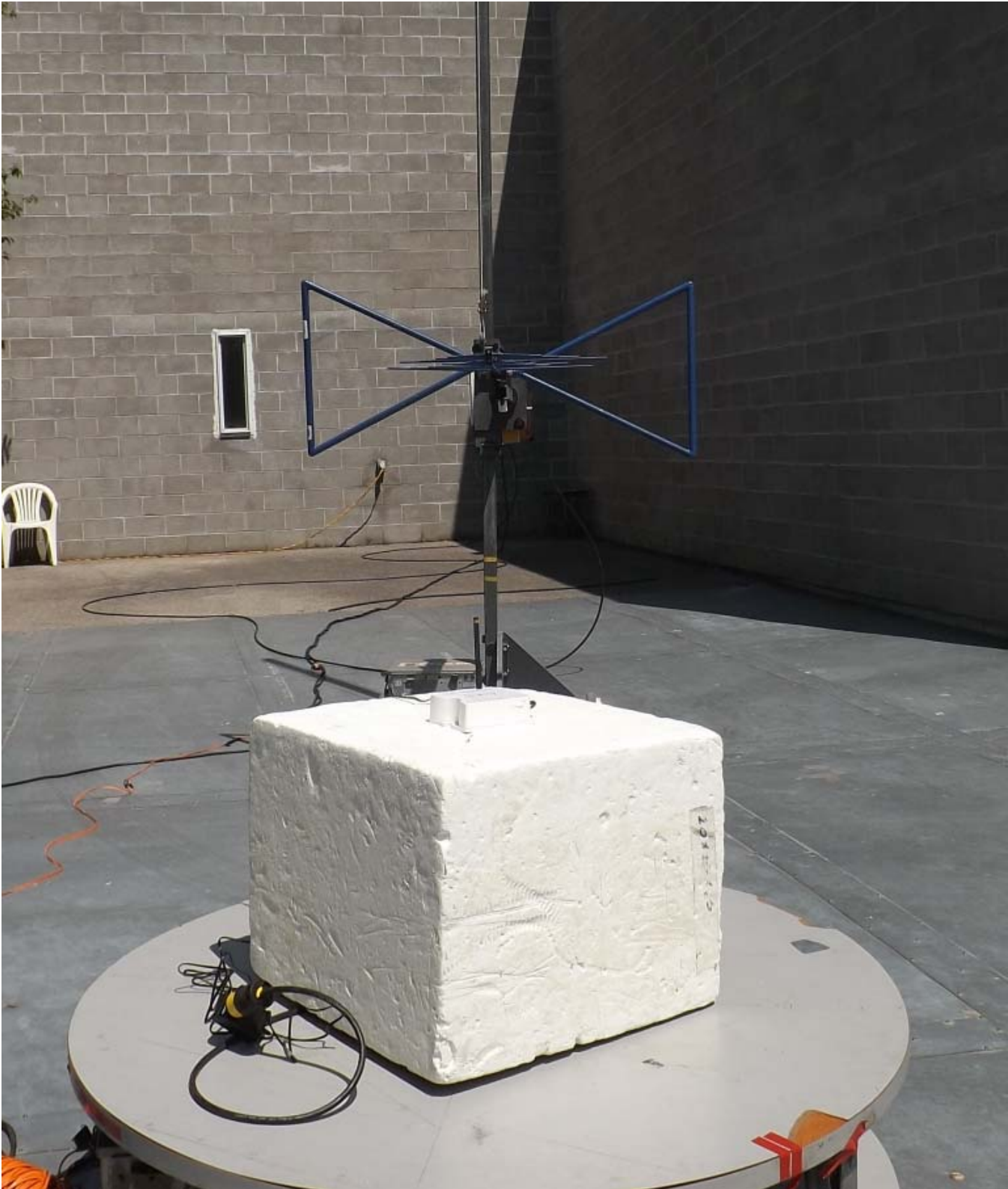
Figure E10.2 – Setup, Radiated Tx and Rx Measurements < 1GHz
