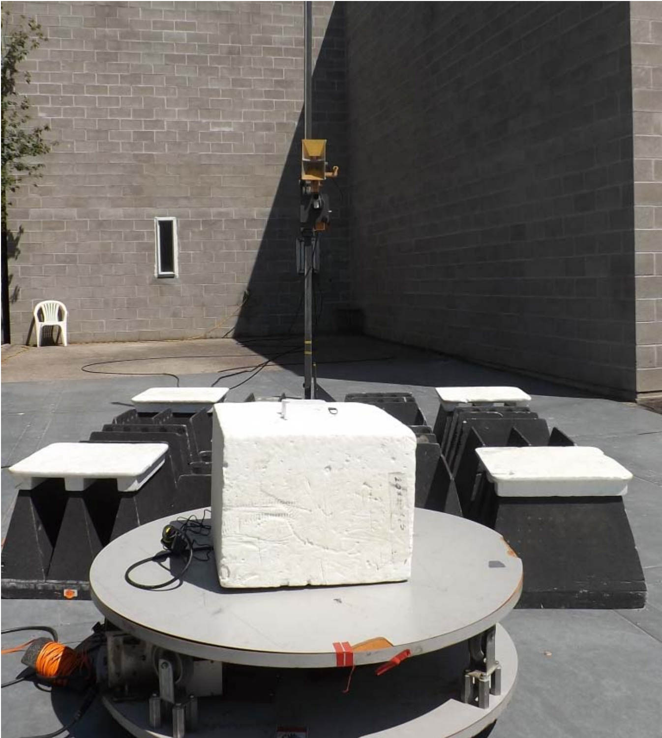
Figure E10.4 – Setup, Radiated Rx Measurements > 1GHz
