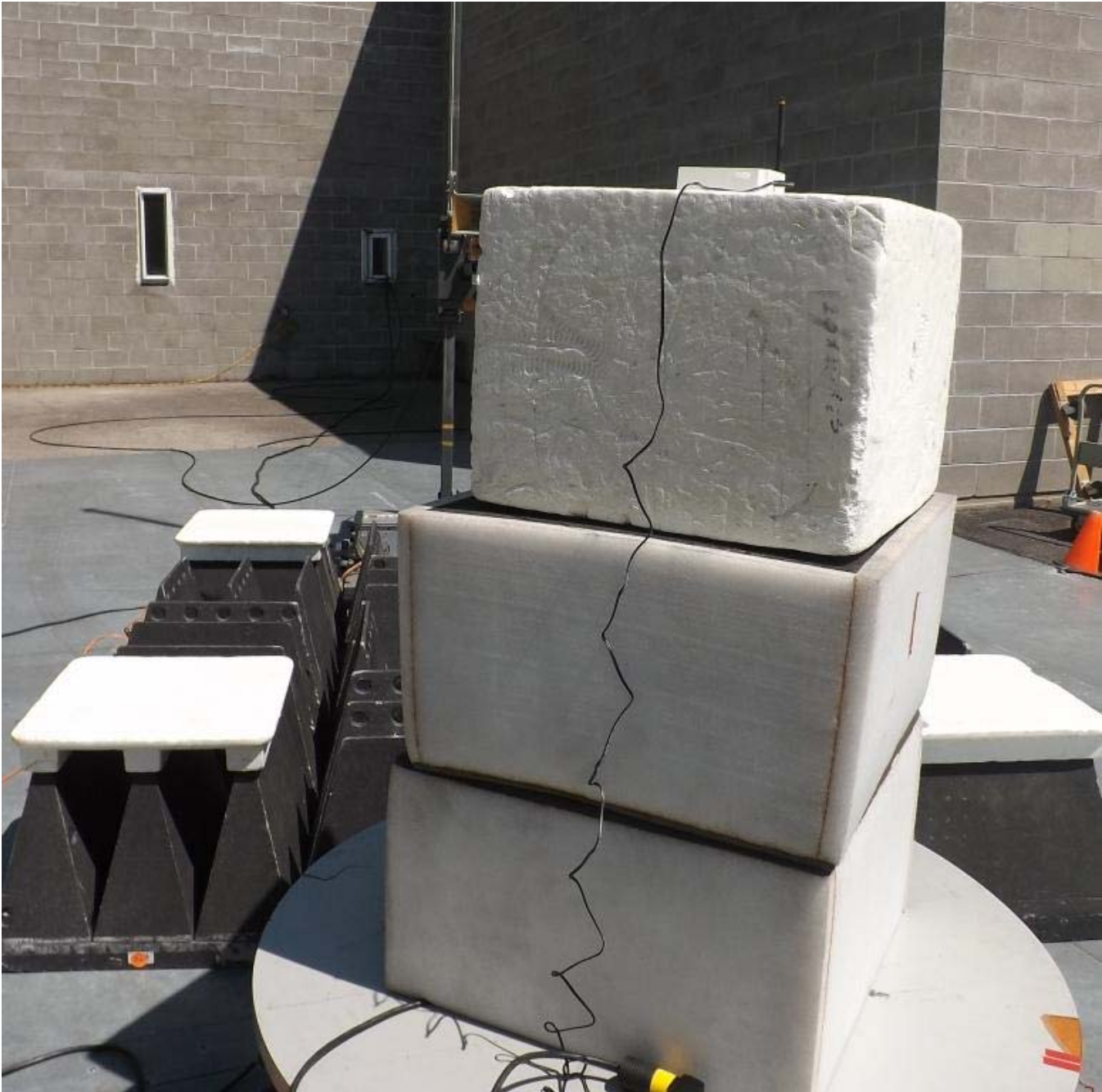
Figure E10.3 – Setup, Radiated Tx Measurements > 1GHz
