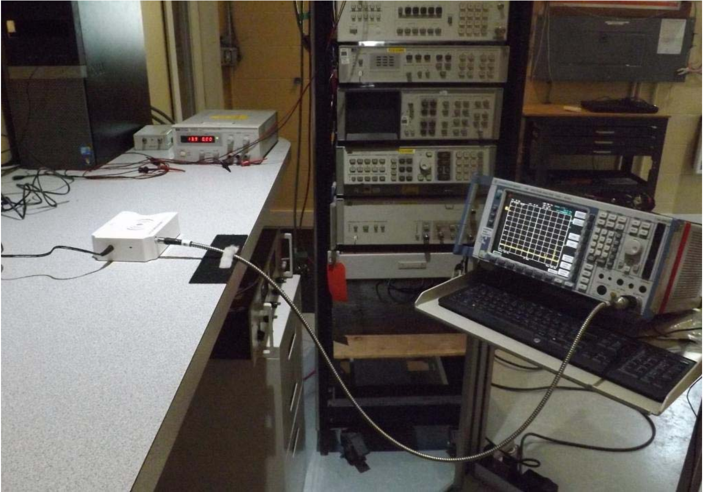
Figure E10.1 – Setup, Conducted Measurements
