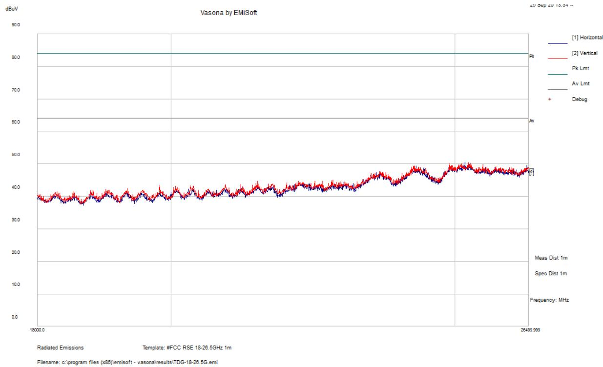
**4) Above 1G Scans (BLE)****1 - 18 GHz, measured at 1 meter**
