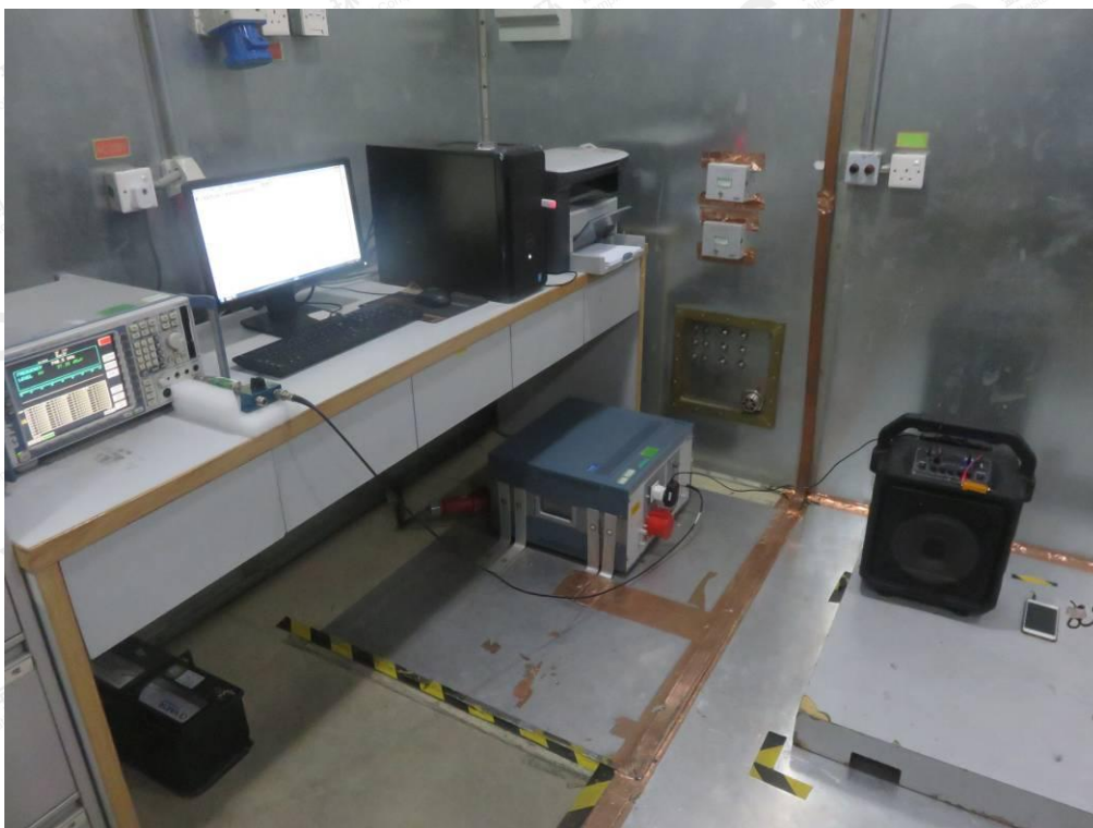
FCC RADIATED EMISSION TEST SETUP
