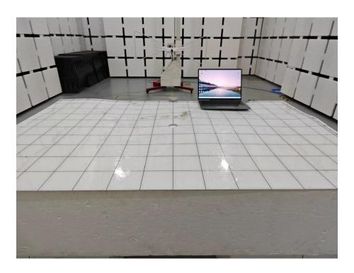
Set-up for Radiated Spurious Emission, Above 1GHz
