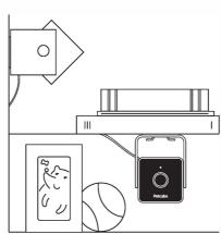
The device can be placed on a wall or a shelf bottom. Petcube Cam comes with a metal plate and a mounting tape. Mount the plate in the desired location and the camera foot will magnetically snap to it. It also works with other metallic surfaces:
