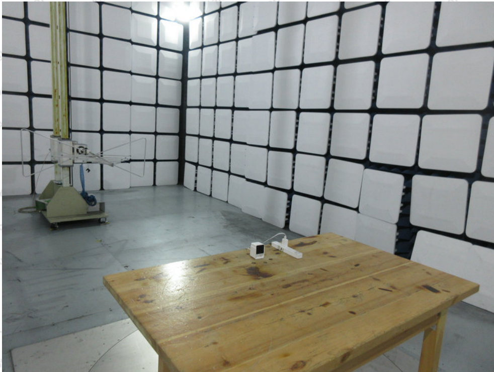
Photo of Radiation Emission Test
