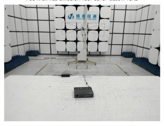
FCC RADIATED EMISSION TEST SETUP ABOVE 1GHZ
