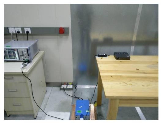
FCC RADIATED EMISSION TEST SETUP BELOW 1GHZ
