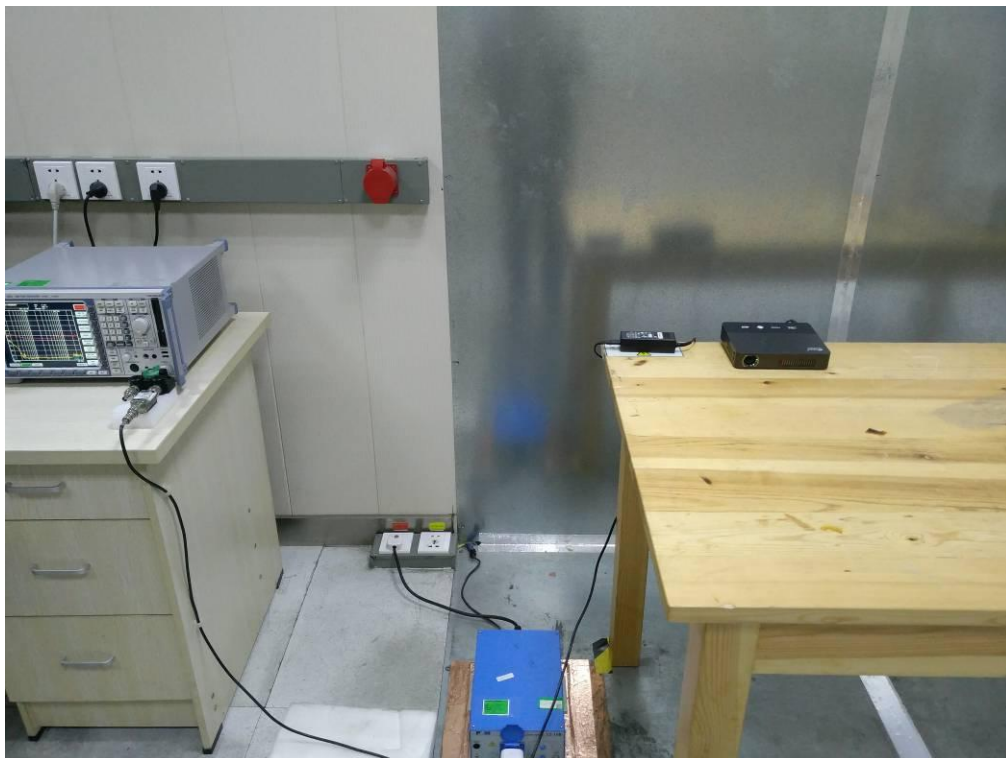
FCC RADIATED EMISSION TEST SETUP BELOW 1GHZ
