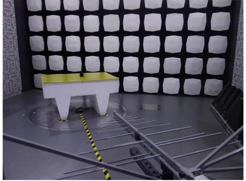
1.2 Radiated Emissions(30MHz-1GHz) Test Setup
