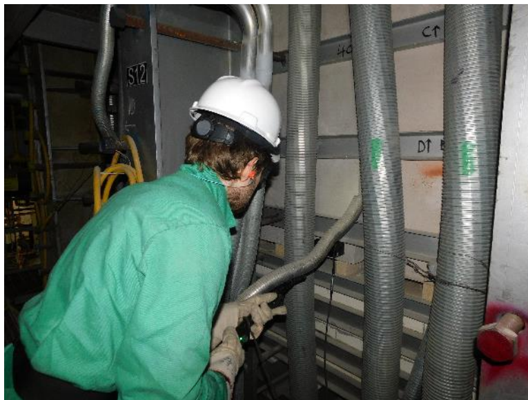
Figure 1 - FTS200 being used to measure sidewall where the FTS400 cannot fit.
