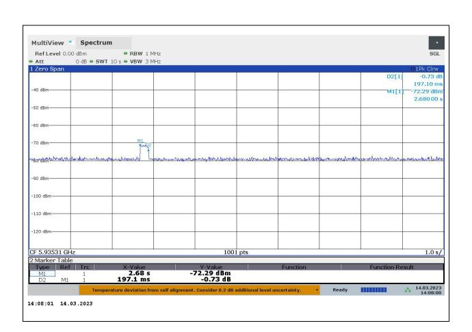
Time denotes total time from the remote button press commanding radar on to button release and radar off. The measured time was 197.1 ms.
