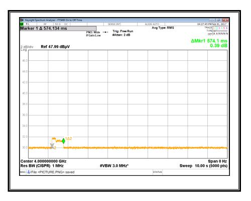
Time denotes total time from button press commanding radar on to button release and radar off. The measured time was 574.1 ms.
