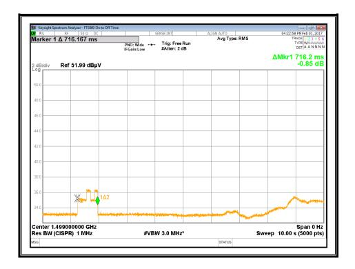
Time denotes total time from button press commanding radar on to button release and radar off. The measured time was 716.2 ms.
